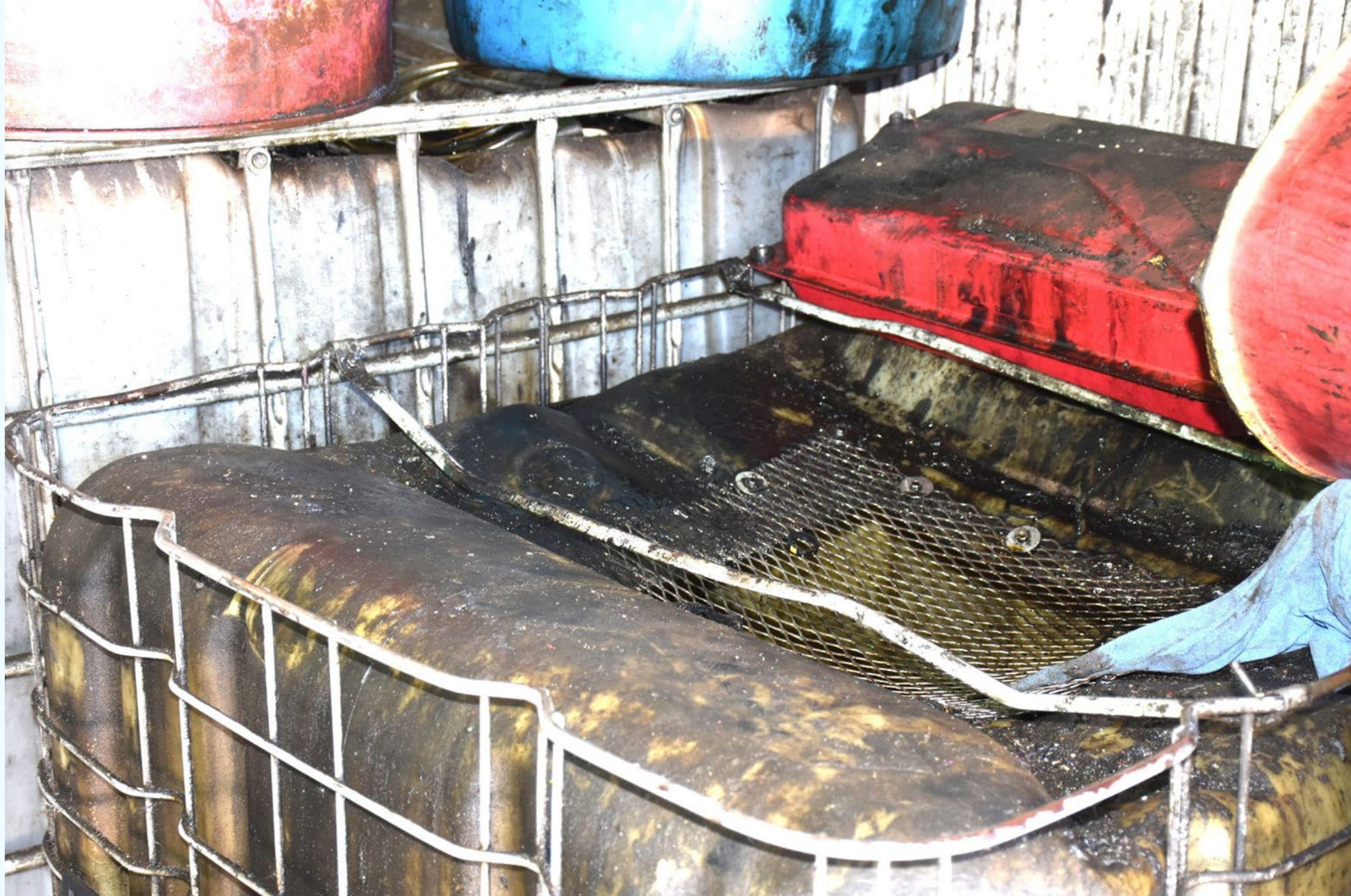
Open drain rack with no means of closing the opening (even when not draining).
